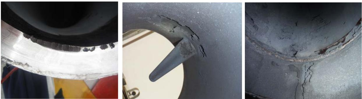
The pictures above show typical consequences of condensation corrosion and in which forms condensation corrosion may occur. Carbamate containing gas condenses on cold spots and the then formed liquid ammonium carbamate does not contain sufficient oxygen so active corrosion instantly starts.
