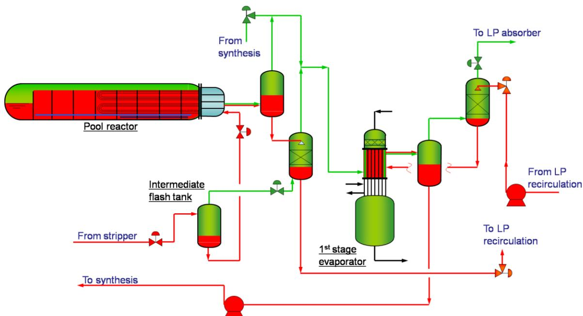
Fig. 6: Flow sheet LAUNCH MELT™ Low Opex Design
