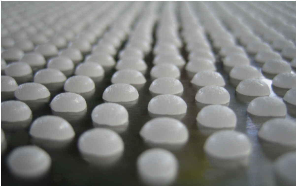
Picture 7: Urea Pastille distribution on the running steel belt (close up)
