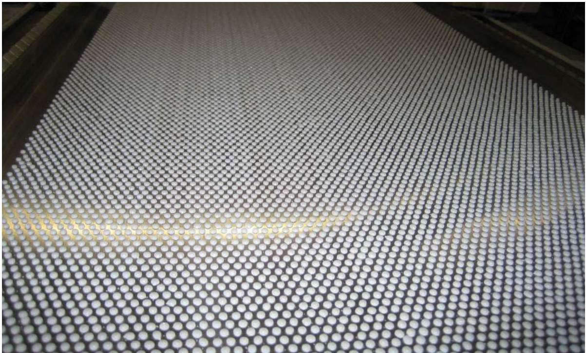
Picture 6: Pastille distribution on the running steel belt.
