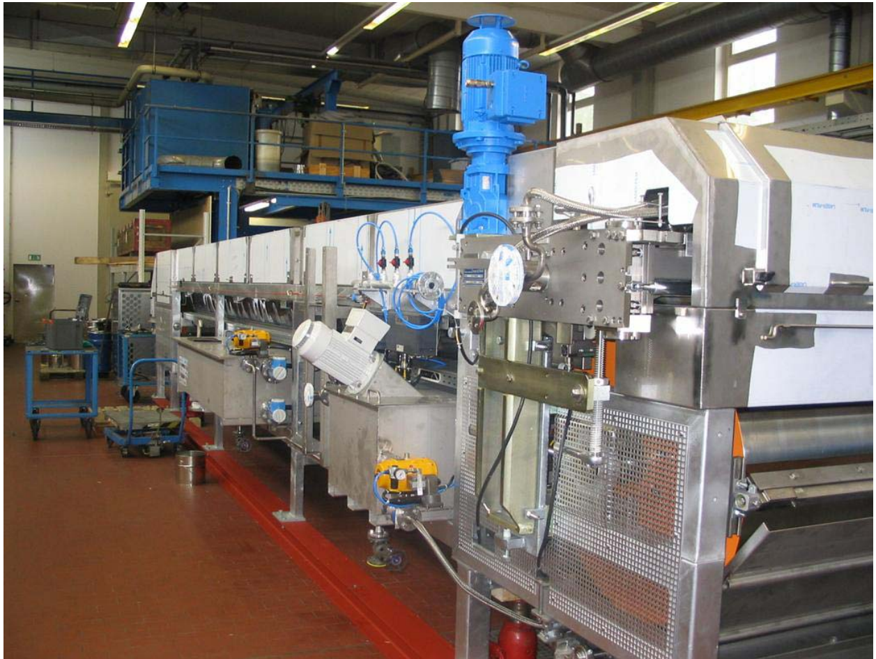
Picture 2: Rotoform skid mounted equipment showing the hood by which the ammonia emissions can easily be caught.
