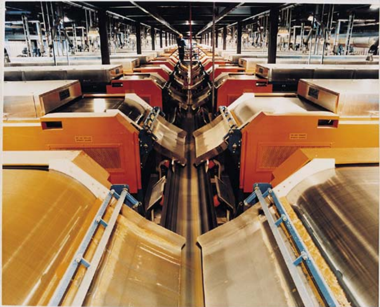
Picture 9: Shell Canada has 46 Rotoformer lines in operation producing 6000 mtpd during 365 days a year
