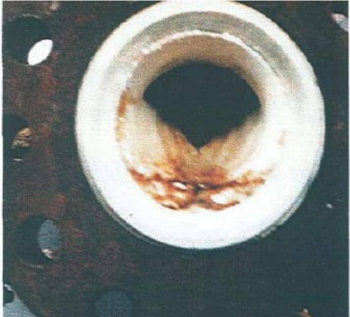
**Figure 5: Clogged outlet line of a ammonium carbamate safety valve**
