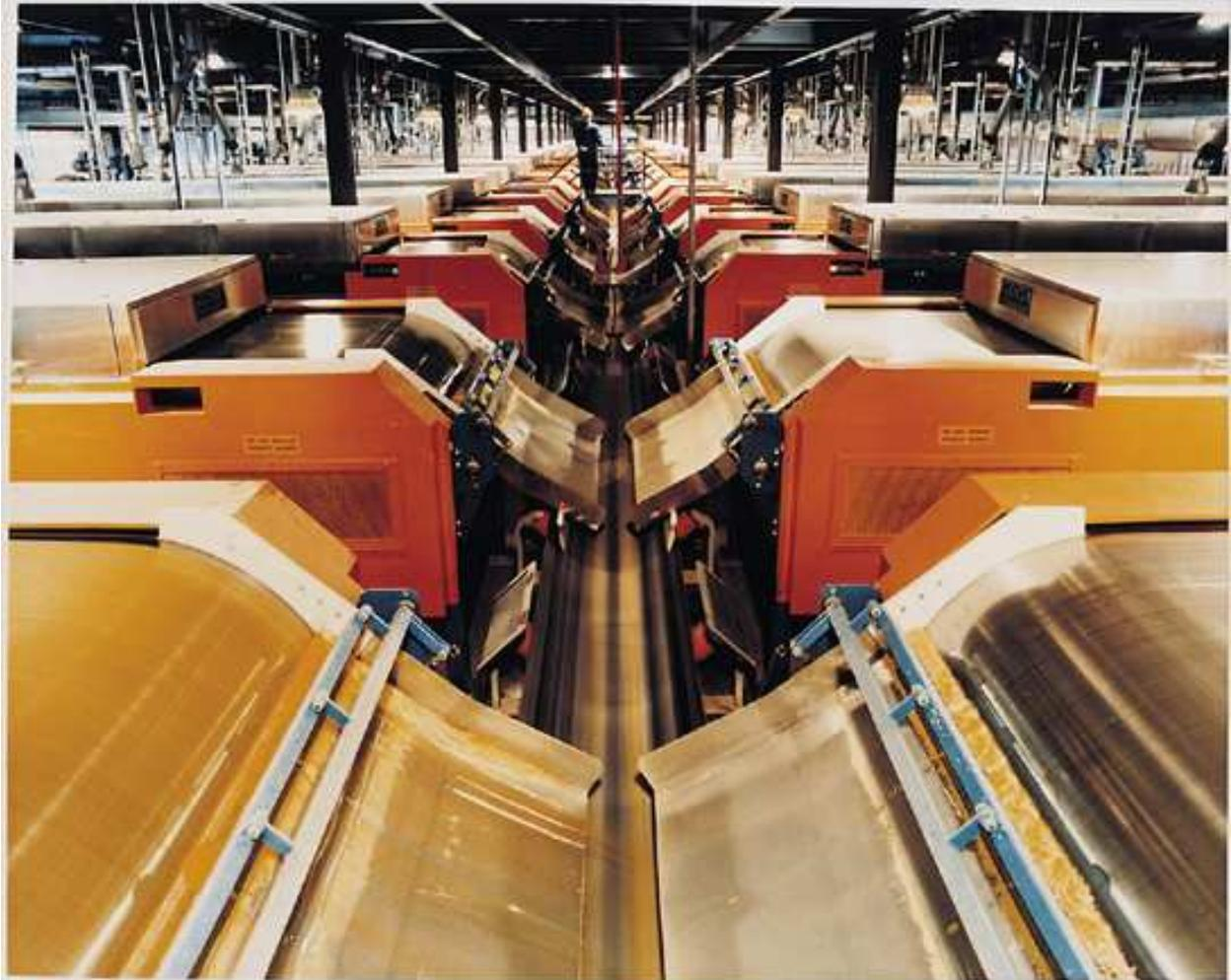
**Picture 3: Shell Canada has 46 Rotoformer lines in operation producing 6000 mtpd during 365 days a year**
